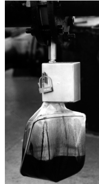
Sampler with valve lock fitted to satisfy PSA guidelines.
