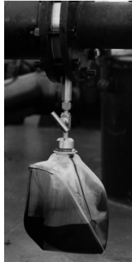
Sampler in use on a Bunker Barge.
