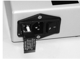
Replace box, ensuring white arrows are aligned.
