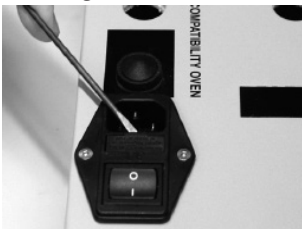
Remove fuse box using a screwdriver.
